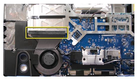
3. Connect the ambient temp sensor cable and the fan cable to the logic board connectors.
